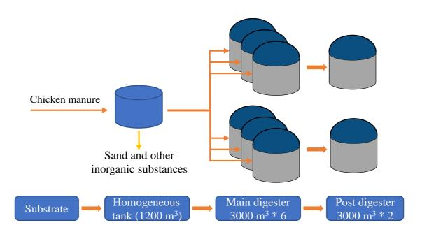
Figure 2: Process flow chart of the first phase of the biogas facility
