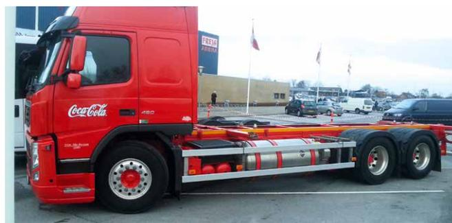
**Figure 3:** Dual-fuel truck that is powered simultaneously by liquefied methane and diesel (dual fuel). The LBG/LNG storage tank is clearly visible on the side of the truck.
