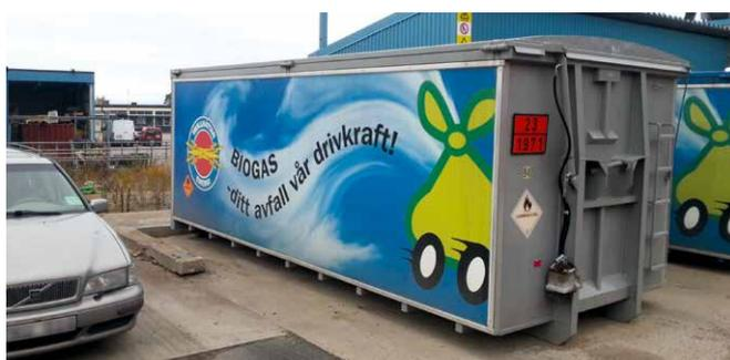
**Figure 4:** Container used for transportation of compressed biomethane in Sweden. The container is filled with high pressure gas cylinders.
