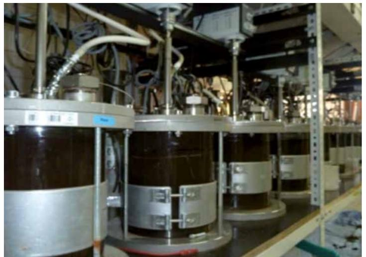
Figure 11: Continuous biogas fermentation at laboratory scale
