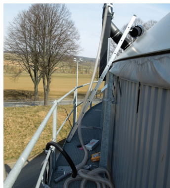
Figure 10: a) Double layer inflated roof (DBFZ) b) measurement setup at a digester (DBFZ)
