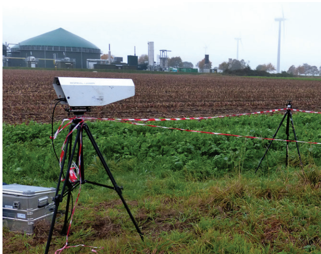
Figure 6 Open path tuneable diode laser systems in use at a biogas plant (DBFZ)
