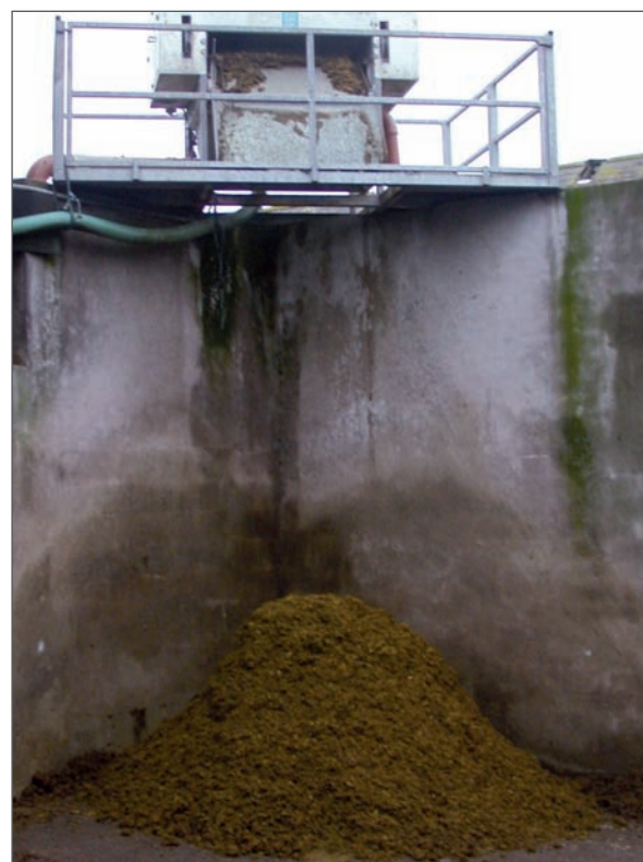
Photo 8: Example of a rotary screen separator producing a stackable fibrous fraction and a free flowing liquid fraction
