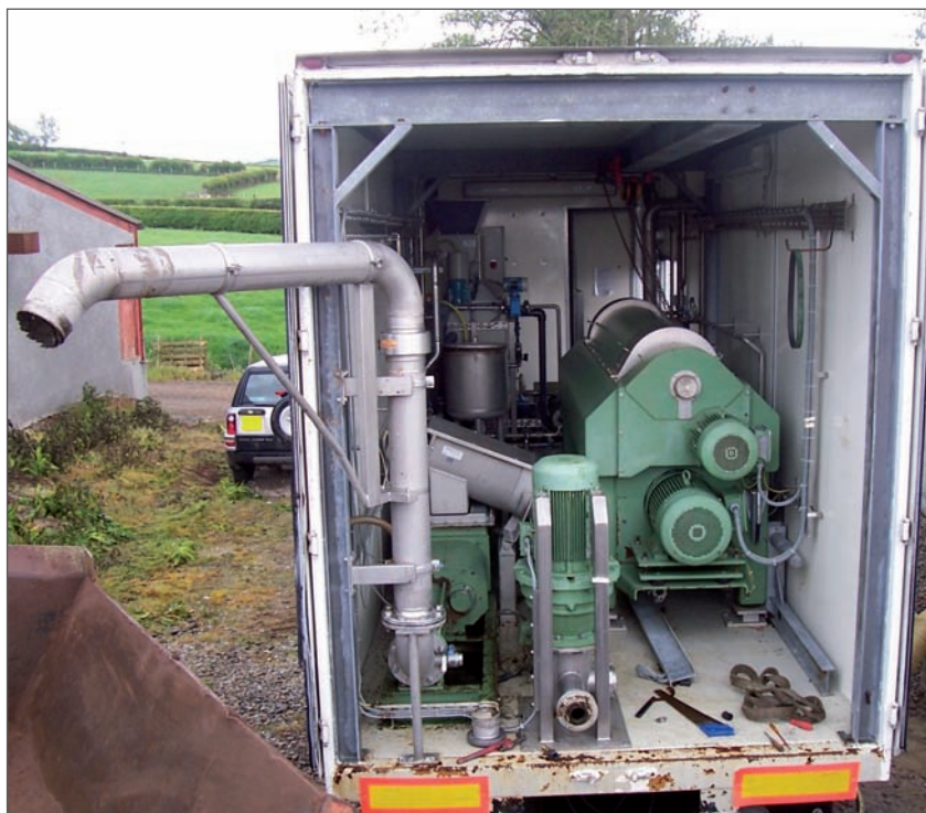
Photo 9: Decanter centrifuge mounted in a trailer unit for use in different locations
