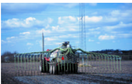
Figure 8. Dragging hoses for the application of digestate Source : BioPress
