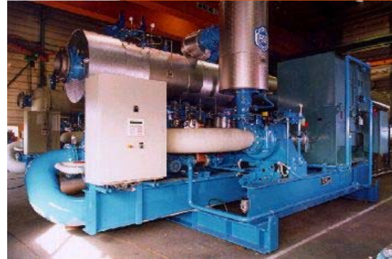
Heat pump for energy recovery, Umea Sweden
