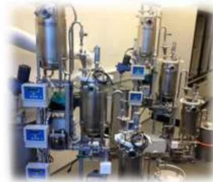
Mini-pilot biogas plant
