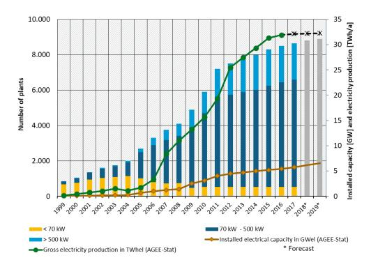
Source: DBFZ,2019. Database: Distribution of biogas plants by plant size on the basis of the DBFZ plant database; installed plant capacity and electricity generation according to AGEE-Stat 2/2019 (UBA 2019), \*DBFZ forecast (modified according to Lenz et al. 2019)
