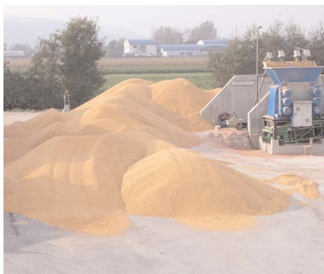
Figure 2: Delivered grains (e.g. maize) are cracked directly before ensiling in the silage clamp silos.
