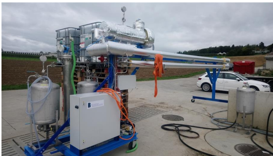
Figure 12.2. Steam Explosion test rig at the Grangeneuve AD Installation. ©BFH
