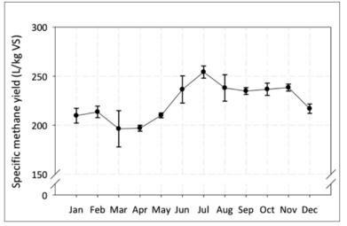
Figure 5: Annual variation in methane potential of L.digitata in the UK in 2008 (adapted from Adams et al., 2011)
