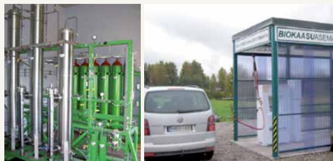
Figure C2 Patented Metener biogas upgrading technology (J. Läntelä) (left) and Kalmari Farm's new fully commercial biogas filling station (O. Pakarinen) (right)
