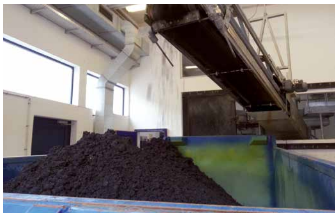
Figure 5: Dewatered sewage sludge
