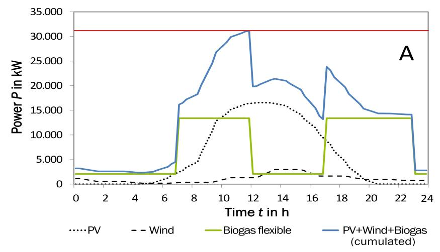
Source: modified based on Trommler et al. 2017: Can Biogas Plants Contribute to Lower the Demand for Power Grid Expansion?, Chem. Eng. Technol. 2017, 40, No. 2, 359–366, DOI: 10.1002/ceat.201600230
