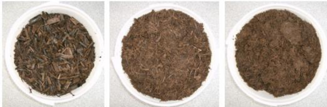
Figure 32 Left: willow without flash; Middle: willow at same conditions with one flash; Right: willow at same conditions with double flash
