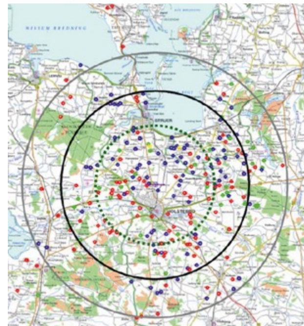
Figure 2: The area of animal slurry collection around the biogas plant, with the average radius of 20 km. Source: Maabjerg BioEnergy
