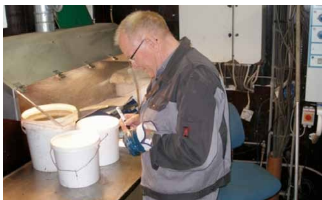
Figure 6: Taking samples for dry matter content analysis of raw slurry and digestate at the biogas plant’s own laboratory (Photo: Linko Gas)
