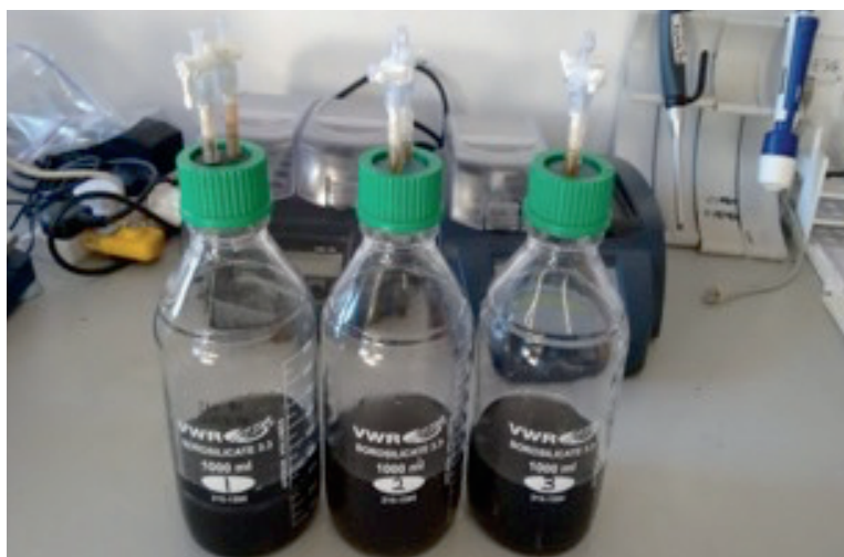
Figure 3.1. Simple experimental examination of ex-situ biological methanation (from Guneratnam et al., 2017)
