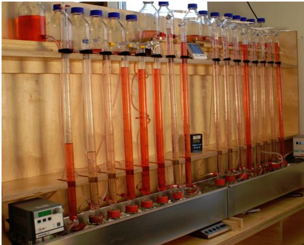
Figure 4 Determination of the biogas potential by Weihenstephaner Biogas Yield Test WBT(R) (Pesta, 2024)
